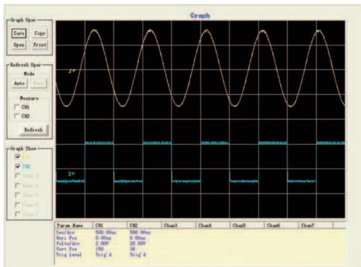
The included Easyscope software provides seamless integration between the oscilloscope and PC. Capture and transfer waveforms, screen images, setups and measurement results to a Windows PC via the USB device port on the back of the instrument.
